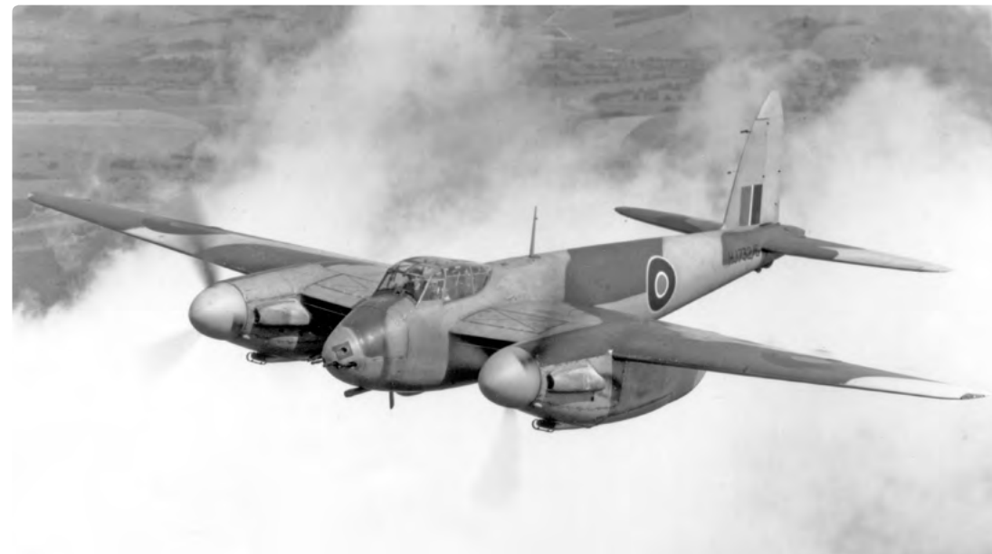
ABOVE In the spring of 1943 de Havilland Mosquito FB.VI HJ732 was modified to carry a single Molins 57mm-calibre gun firing 6lb shells, the barrel of which is seen here protruding from the underside of the nose. The installation of the Molins plus the four Browning 0.303in machine-guns retained from the Mosquito fighter variants is seen OPPOSITE .
