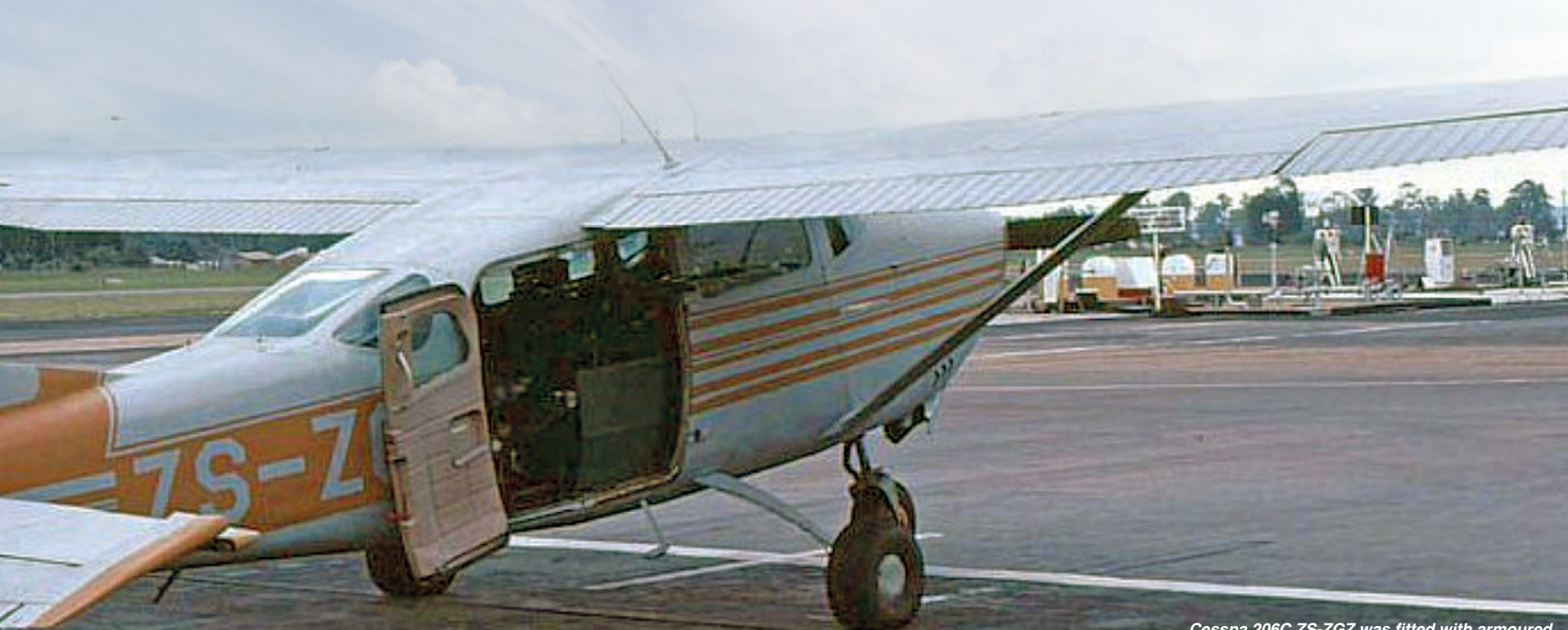
Cessna 206C ZS-ZGZ was fitted with armoured seats and a single machine-gun mounted in the open doorway. Note also the bulletproof shield. Stored behind the closed rear cargo door would be 3,000 rounds of belted ammunition. Matt-orange paint has been applied over the anti-SAM grey to provide a civilian appearance ahead of the arrival of the international election monitoring force in December 1979.
